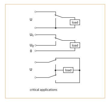
Inflammable gases in the ambient atmosphere may be ignited by the arc at the relay contacts. Even with sealed relays, the case seal does not prevent the penetration of combustible gases into the relay.
